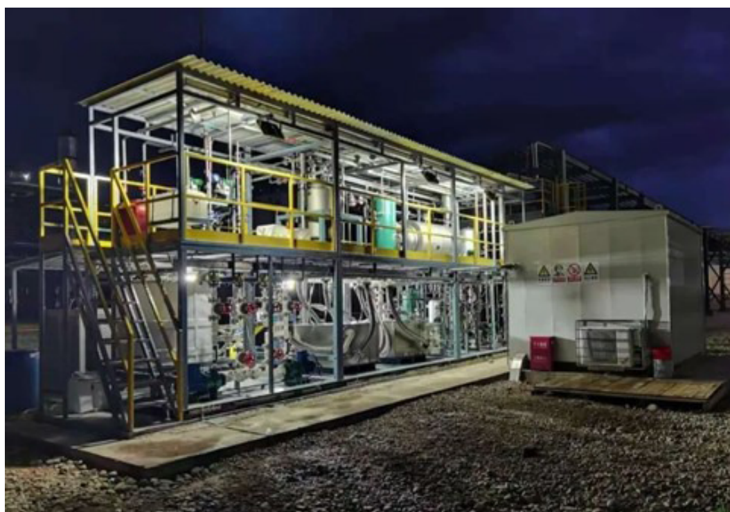
Fig. 12. The demonstration system of \text{CO}_2 electrolysis for syngas production [Reprinted from (Carbon Energy Technology Co. LTD, 2020)].
