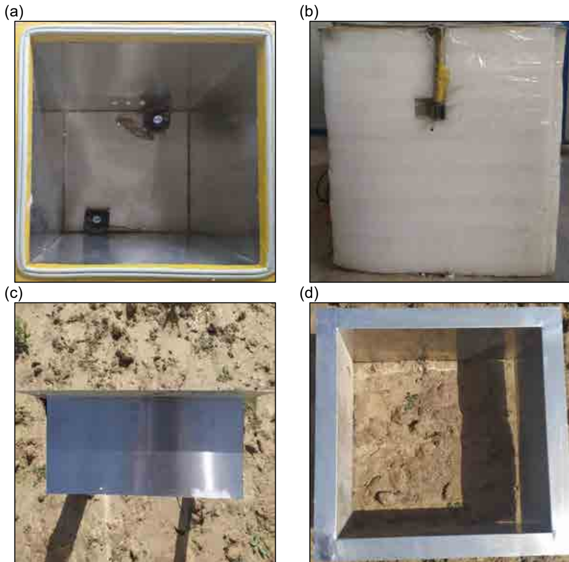
Fig. 4. Photographs of the chamber: (a) top view and (b) side view of the sampling chamber; (c) side view and (d) top view of the stainless steel base.
