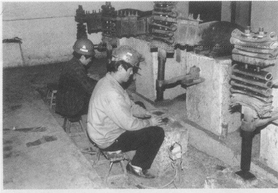
Fig.7 Cutting the thinner gold block into small square parts.
