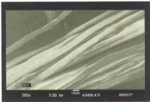
图 9 加固后老化丝的扫描电镜图 Fig.9 The SEM image of silk samples after consolidation
