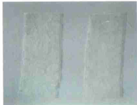
图 12 水解老化样品 左. 加固后, 右. 加固前 Fig.12 The hydrolyzation-aged sample Left: after consolidation Right: before consolidation
