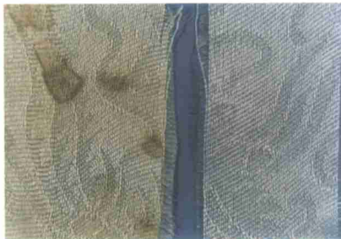
图 13 霉菌试验 左. 加固前, 右. 加固后 Fig.13 The mildew experiment Left: before consolidation Right: after consolidation
