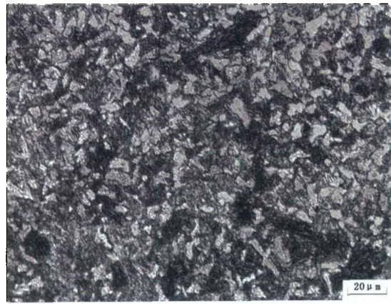
图 6 样品呈 1 铜柄铁刃剑刃部金相组织 Fig. 6 The microstructure of the blade of iron blade sword with bronze handle
