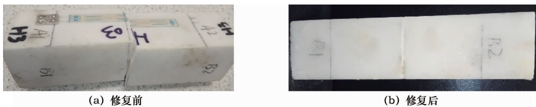
图7 贯通裂缝石梁修复前后的石梁外观对比图 Fig.7 Appearance comparison of the marble beams with through cracks before and after restoration
