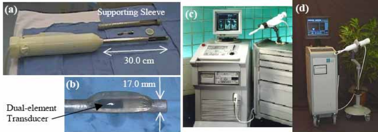
FIGURE 4. (a) The computer-controlled laparoscopic HIFU probe and the supporting sleeve, (b) a close-up of the probe tip covered with the supporting sleeve and the water-filled latex sheath, (c) Sonablate ® 200 HIFU device, and (d) Sonablate ® 500 HIFU device.
