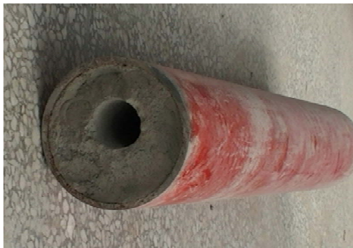
图9 钻孔结束后的围岩相似材料 Fig.9 Simulated material of surrounding rock after borehole drilling
