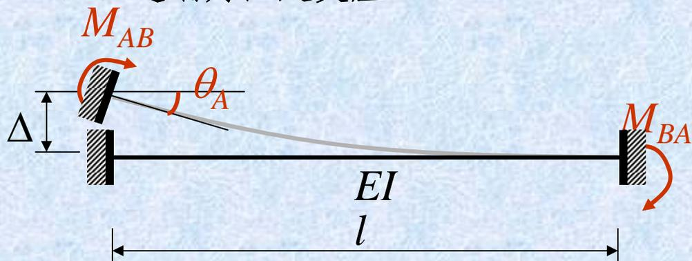
$$\left. \begin{aligned} M_{AB} &= 4i\theta_A + 2i\theta_B - 6i\frac{\Delta}{l} \\ M_{BA} &= 2i\theta_A + 4i\theta_B - 6i\frac{\Delta}{l} \end{aligned} \right\} \dots\dots(1)$$
