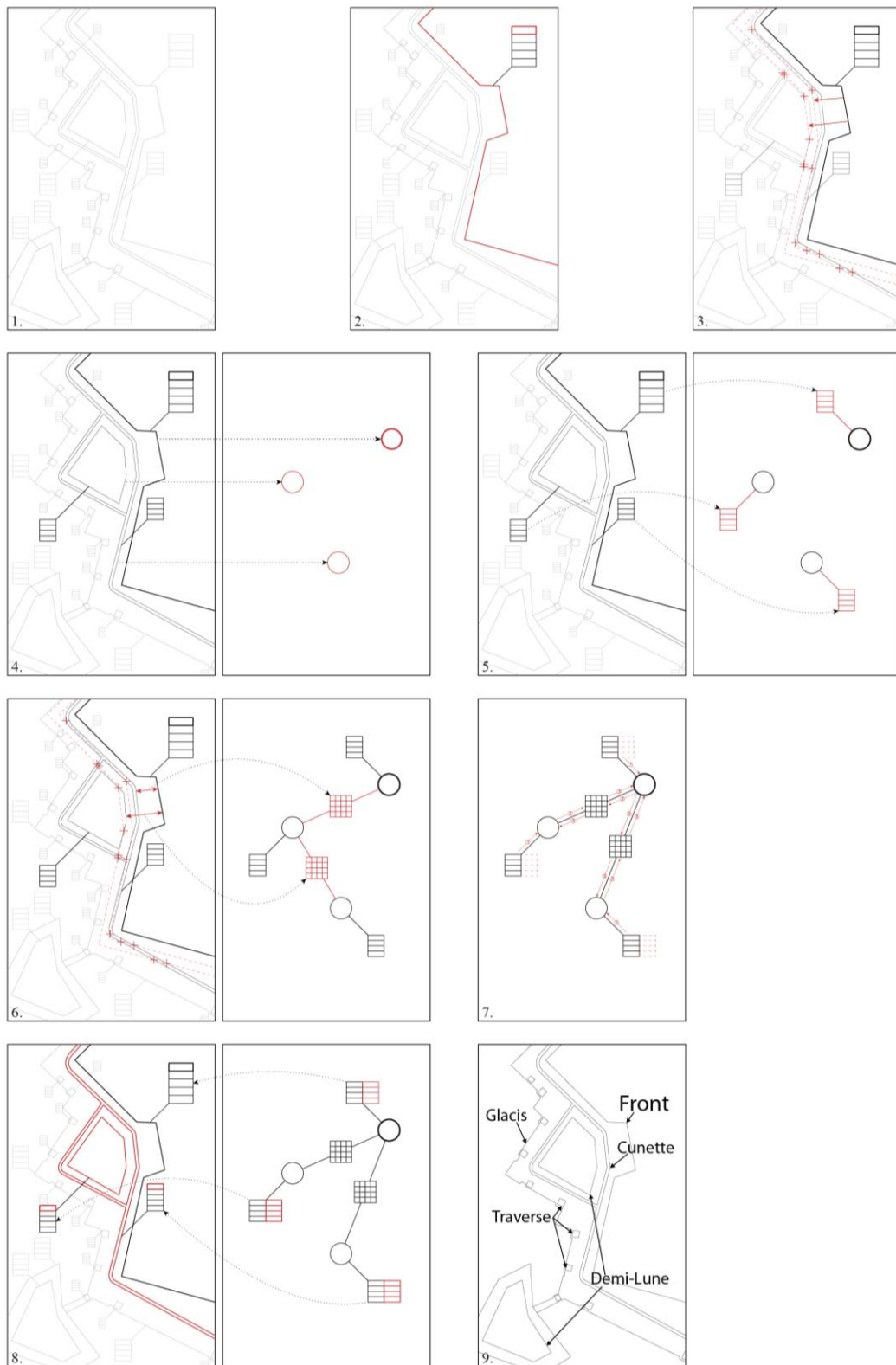
Figure 7. Consistency Evaluation Heuristic, identification of military architectural elements according to the morphology of the architectural system using a factor-graph abstraction and inference based on loopy belief propagation 1: Segmented geometry. 2-3: Propagation from the bastioned front (core fortification system element). 4: abstraction of the segmented geometry in nodes (variable vertices). 5: Adding unary factor vertices from precomputed geometric evaluation. 6: Adding binary factor vertices from the theoretical relations 7-8: Message passing via belief propagation 9: Identification, Semantisation
