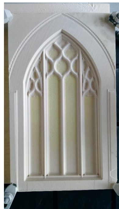
Figure 3: Milling process showing layer of glue.
