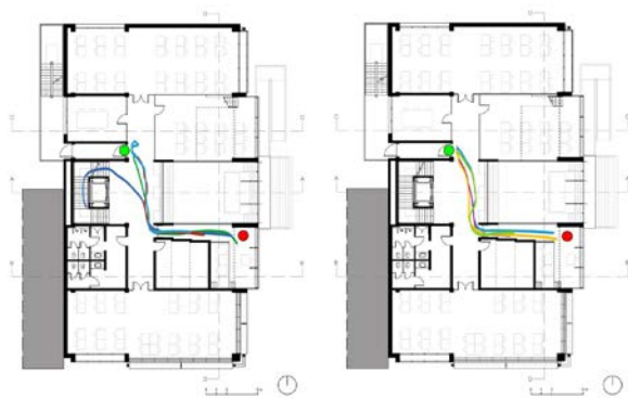
Figure 14: Path-finding for the Target 5 (emergency exit) in the refurbished building, left without signposting, right with signposting.
