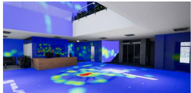
Figure 11-12: The entrance of the refurbished building and its eye-tracking analysis from one test.
