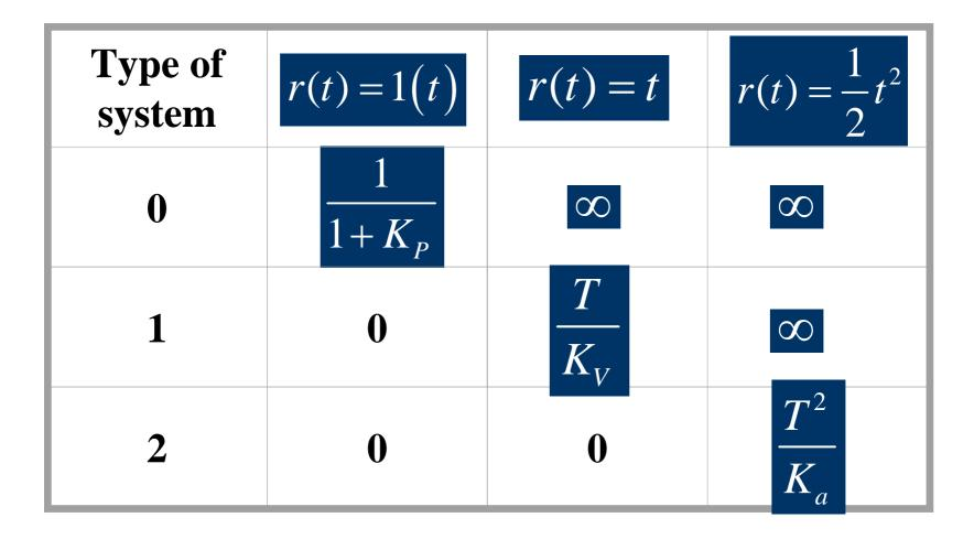
Example: The structure of discrete system is shown in the figure with sampling period T=0.1s. Obtain steady-state error under unit step, unit ramp and unit parabolic input respectively.
