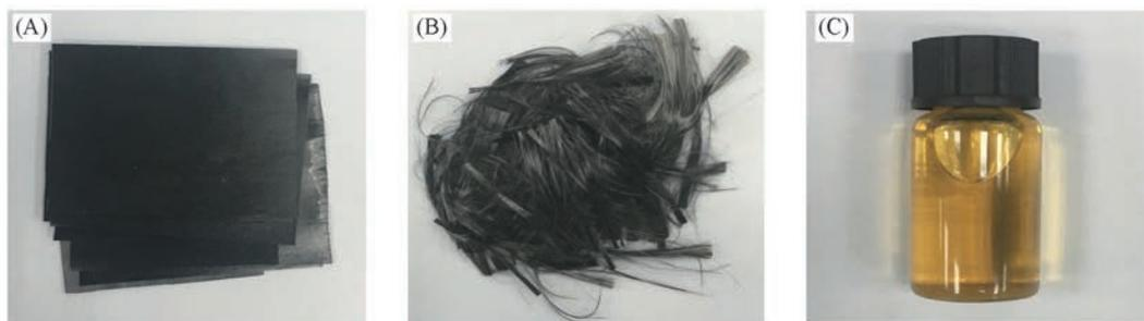
Fig.1 CF/EP before degradation and products after degradation
