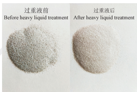
图2 样品过重液前后对比 (照片由曾雪真提供) Fig.2 Samples comparison chart before and after heavy liquid treatment (pictures provided by Zeng Xuezheng)
