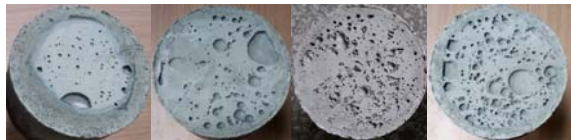
图 10 A 组试件的砂浆界面形态 Fig.10 Mortar interface morphologies of group A specimens
