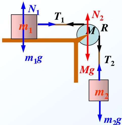
$$\begin{aligned} m_2g - T_2 &= m_2a \\ T_1 &= m_1a \\ T_2R - T_1R &= J\beta \\ J &= \frac{1}{2}MR^2 \quad a = R\beta \end{aligned}$$
