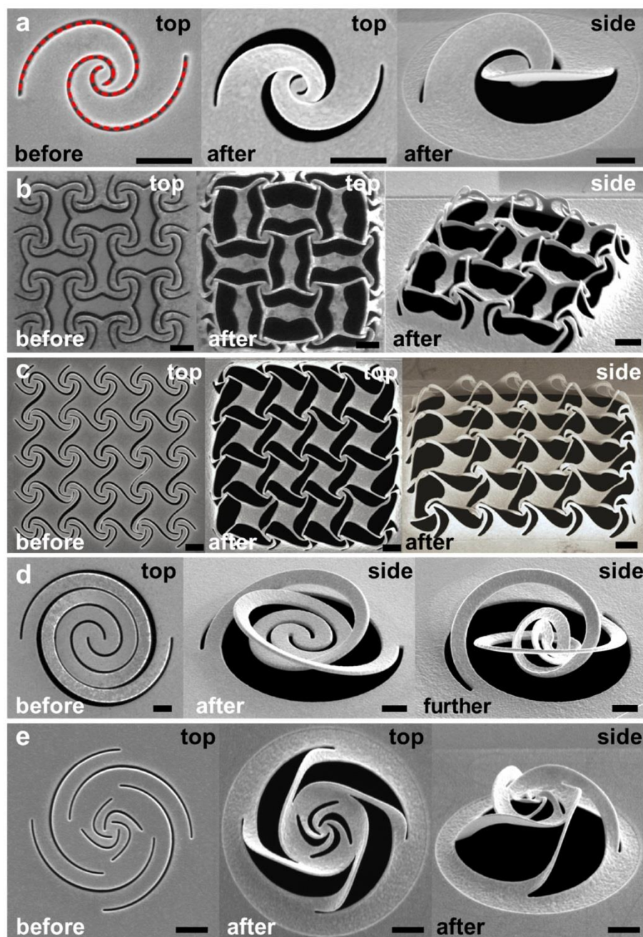
Fig. S2. Exotic 3D structures fabricated by nano-kirigami. Top-view and side-view scanning electron/ion microscope (SEM) images of the typical structures before and after global ion-beam irradiation. (a) Combined double Fibonacci spirals. (b) and (c) Window-decoration-type interconnected nano-barriers. (d) A deformable spiral before and after global ion-beam illumination with different ion doses. (e) A combined spiral heterostructure. Scale bars: 1 \mu\text{m} .
