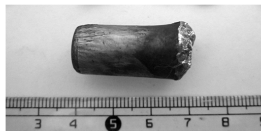
Fig. 9 Shape of projectile after perforation of back skin
