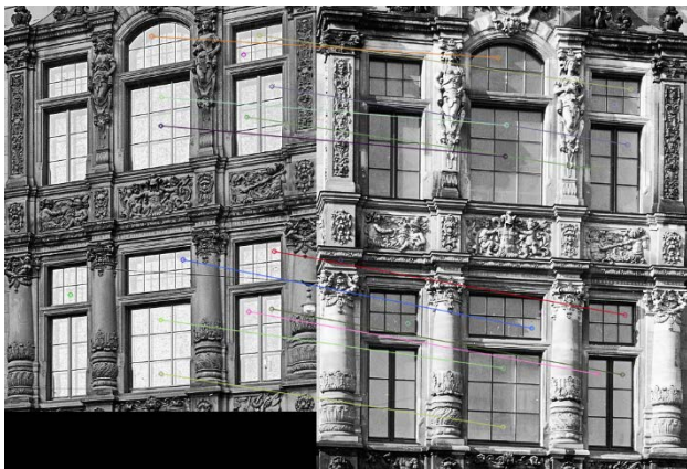
Figure 8. Matched point after calculation of fundamental matrix and filtering using RANSAC for k \in [7,70]
