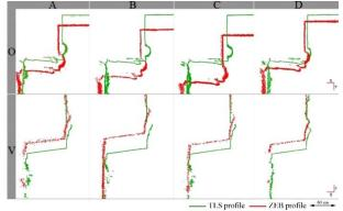
Figure 10. Configuration II, single local alignment. Misalignment errors detected in opposite corners in case of the single local point alignment, related to the O and V areas, pinpointed in Figure 9, according to the processing steps A, B, C, D: O in the horizontal slice, V in the vertical slice.
