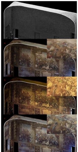
Figure 13. ZEB Point clouds with associated radiometric values: *top*, ZEB point cloud in shaded view. Photogrammetric point clouds: *a*, ZEBcam; *b*, Sony ILCE; *c*, steadicamera. For each point cloud model, a zoomed view of the image used in the photogrammetric process.
