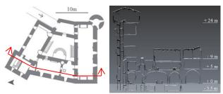
Figure 5. Section of the complexity in the vertical articulation of the Rocca apartments, from multiple ZEB scanning data (right). Schema of the ground floor of the Rocca, in red line, the vertical section (left).
