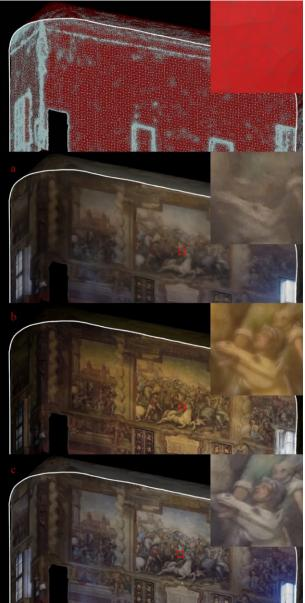
Figure 14. Triangulated surface generated by ZEB point clouds with associated photogrammetric texture. *top*, ZEB triangulated mesh in wireframe view. Texture from: *a*, ZEBcam frames; *b*, Sony ILCE images; *c*, steadicamera frames. For each textured mesh model, a zoomed view of about 50x50cm.
