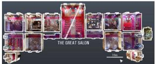
Figure 3. A plan of the complete LiDAR point cloud in the first floor of the Valentino Castle (the cloud is cut at + 2.5 m above the pavement). (Image by LabG4CH, Polito)
