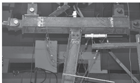
(c) 试件RWUF-1.4边柱Z3弯曲
