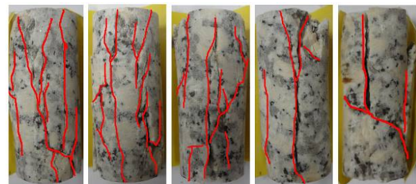
\sigma_3 = 0 MPa \sigma_3 = 10 MPa \sigma_3 = 20 MPa \sigma_3 = 30 MPa \sigma_3 = 40 MPa (b) 花岗岩
