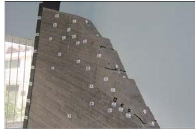
(b) 试验步 8~16( $K_c = 1.105 \sim 1.173$ )模型破坏形态
