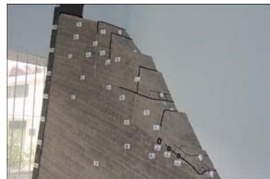
(c) 试验步 17~26( $K_c = 1.181 \sim 1.313$ )模型破坏形态
