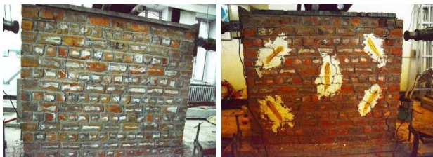
图 10 5-S1 墙体破坏照 Fig.10 5-S1 wall damage photos
