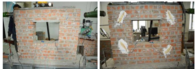
图 12 6-S2-RRBB1 墙体破坏照 Fig.12 6-S2-RRBB1 wall damage photos
