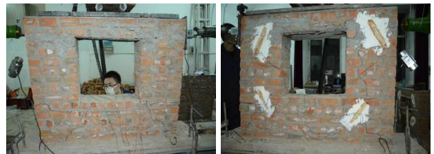
图 18 9-C2-RRBB1 墙体破坏照 Fig.18 9-C2-RRBB1 wall damage photos
