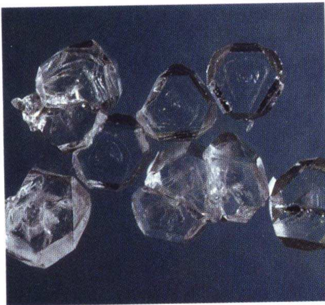
▲ Figure 7.28 Crystals of \text{XeF}_4 , which is one of the very few compounds that contain a group 8A element.
