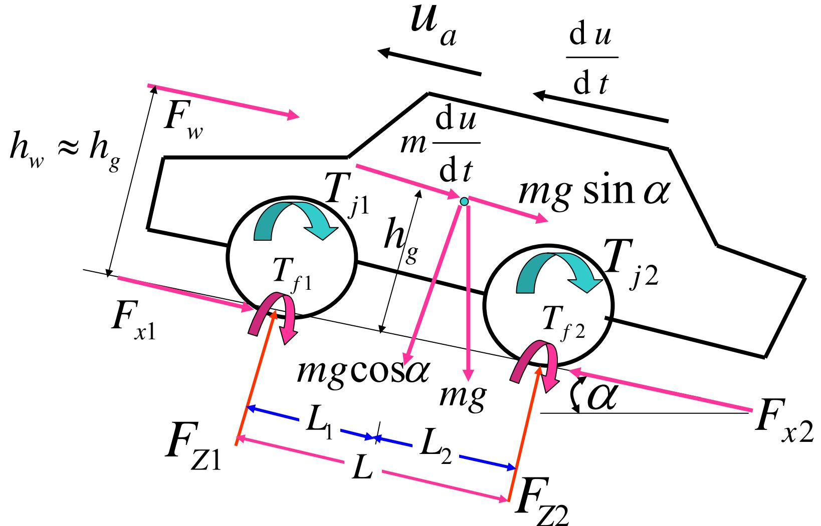
$$F_{Z1}L + \Sigma T + F_w h_w + m \frac{du}{dt} h_g + h_g mg \sin \alpha - L_2 mg \cos \alpha = 0$$
