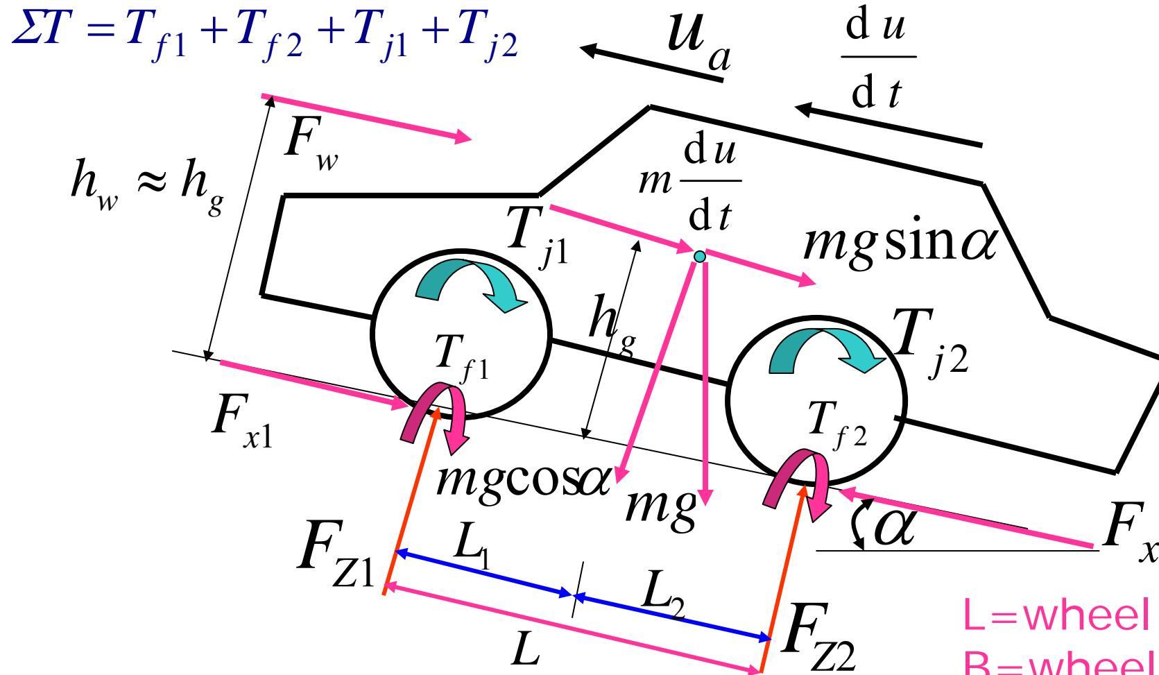
$$F_{Z2}L - \Sigma T - F_w h_w - m \frac{du}{dt} h_g - h_g mg \sin \alpha - L_1 mg \cos \alpha = 0$$
