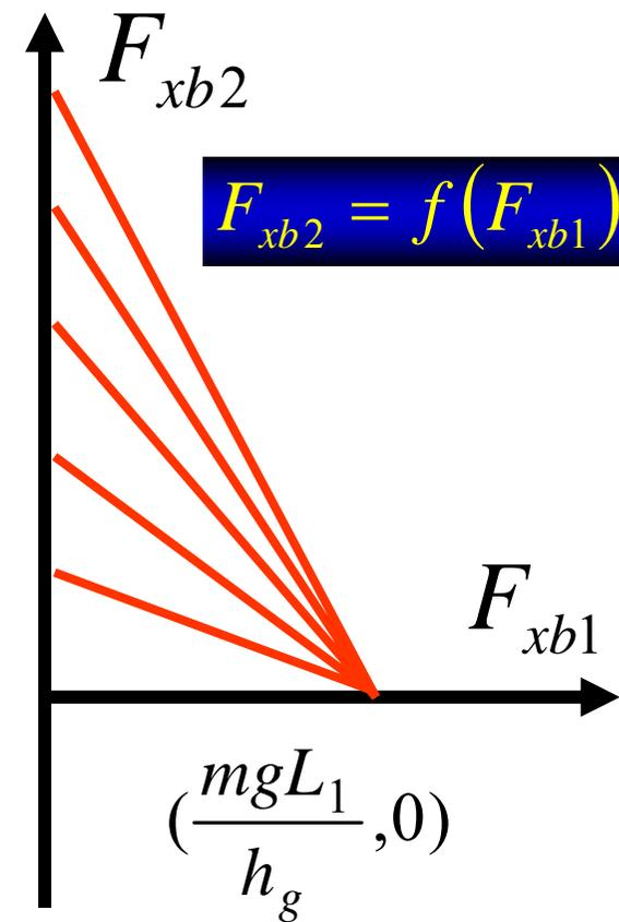
$$F_{xb2} = \frac{\varphi mgL_1}{L + \varphi h_g} - \frac{\varphi h_g}{L + \varphi h_g} F_{xb1}$$
