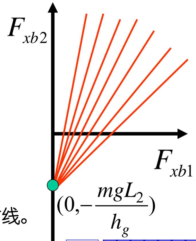
$$F_{xb2} = \frac{L - \varphi h_g}{\varphi h_g} F_{xb1} - \frac{mgL_2}{h_g}$$
