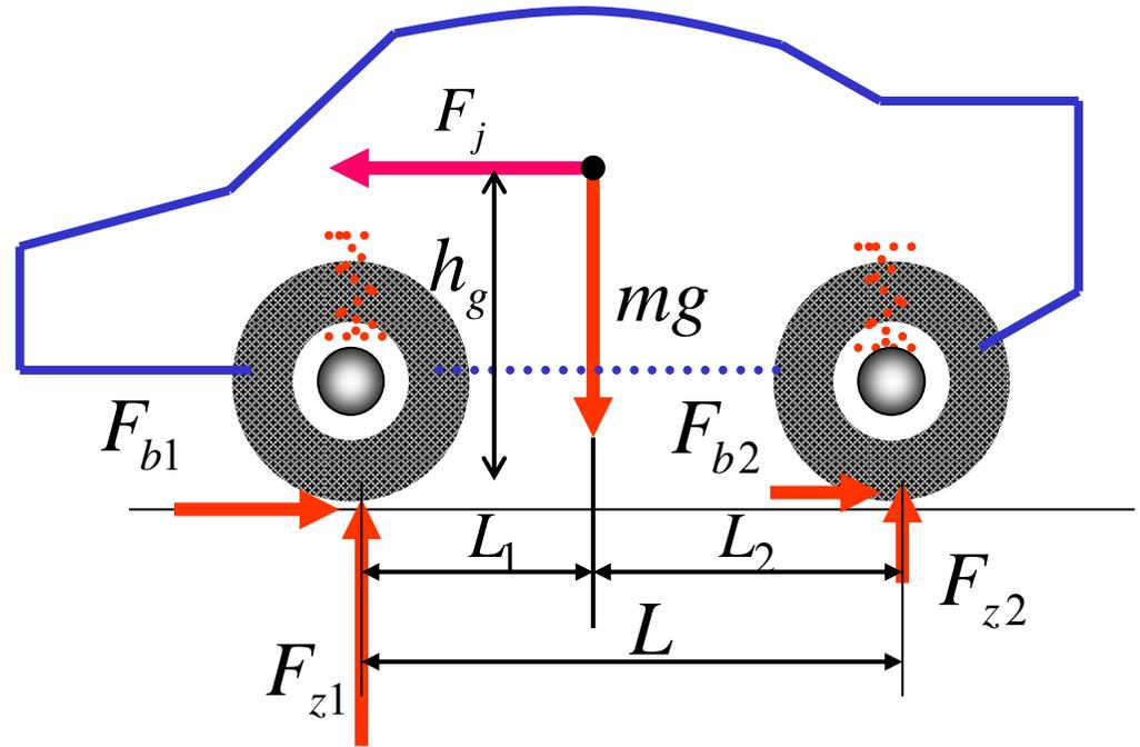
$$F_{z1} = \frac{mg}{L} \left( L_2 + \frac{h_g}{g} \frac{du}{dt} \right) = \frac{mg}{L} (L_2 + h_g \varphi_b) = F_{z10} + \Delta F$$
