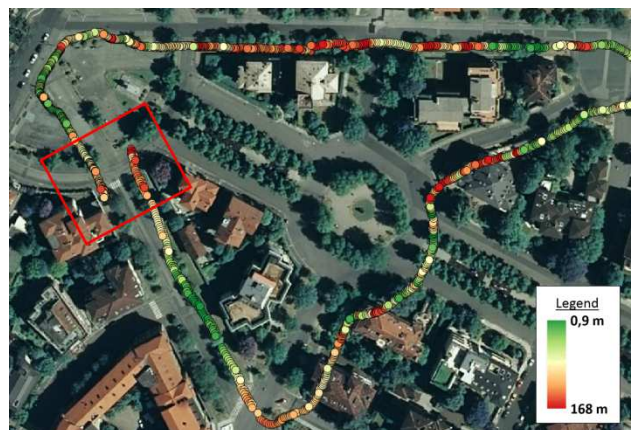
Figure 15. Difference between image coordinates measured by the U-blox 8T and the camera positions estimated by the software Agisoft Photoscan.
