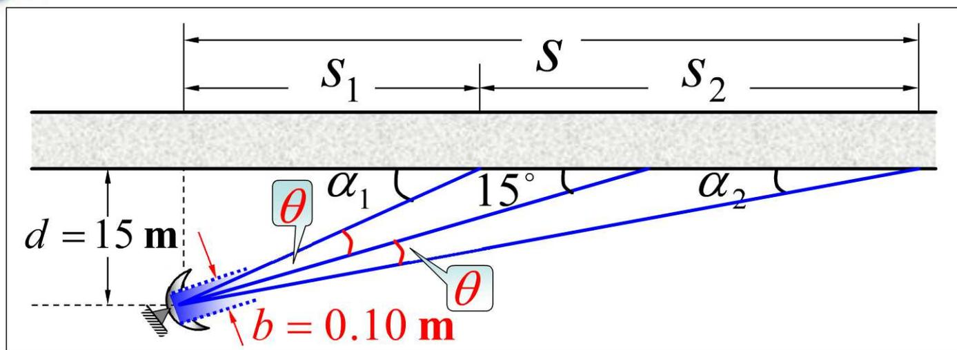
根据暗纹条件  $b \sin \theta = \lambda$ ,  $\theta = \arcsin \frac{\lambda}{b} = 10.37^\circ$
