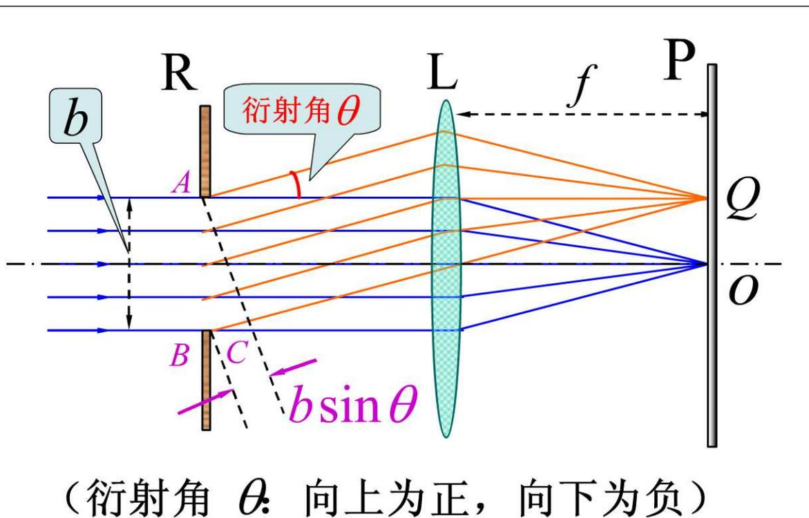
菲涅耳波带法  $BC = b \sin \theta = \pm k \frac{\lambda}{2} \quad (k = 1, 2, 3, \dots)$
