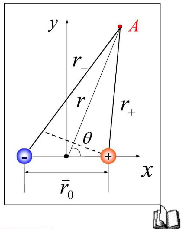
$$\because r_0 \ll r \quad \therefore r_- - r_+ \approx r_0 \cos \theta \quad r_- r_+ \approx r^2$$
