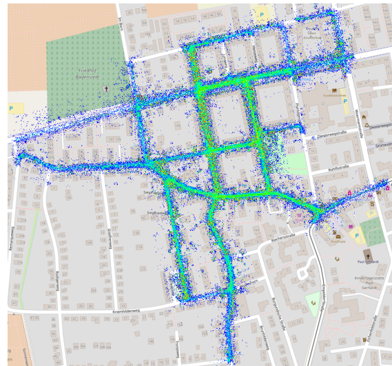
Figure 2. Measurement area in Hannover-Badenstedt (Germany). The scan points are colored by the maximum height difference in every grid cell, from blue (0 cm) to red (2 cm).
