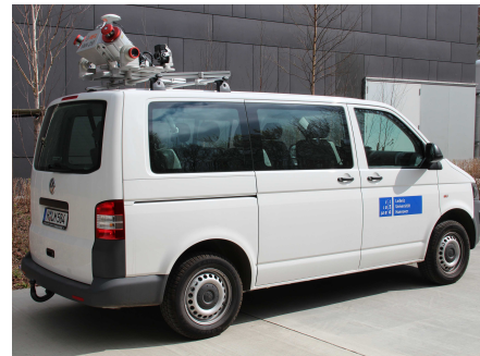
Figure 1. Riegl VMX-250 placed on a Mobile Mapping van.
