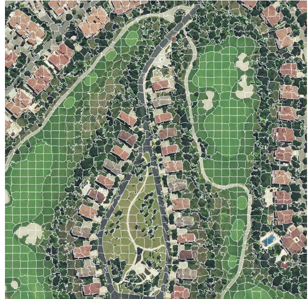
Figure 2. Orthophoto after SLIC superpixel segmentation
