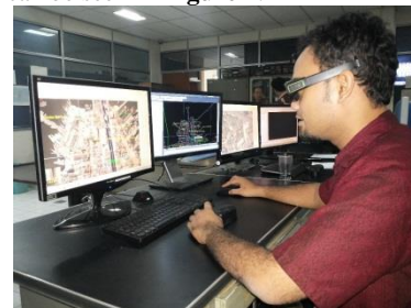
Figure 4. Stereo plotting process (picture taken from Center of Topographic Mapping and Toponym presentation)
