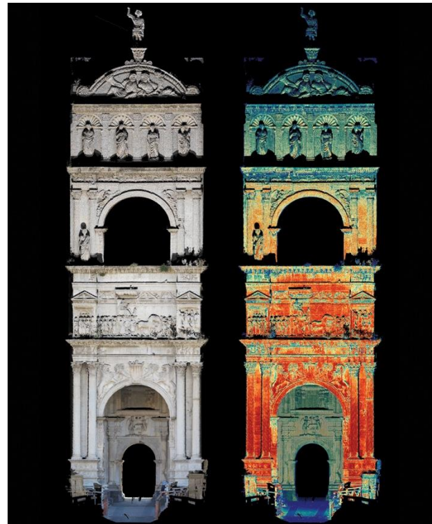
Figure 14. Orthoprojection of the Aragonese arc dot cloud with actual RGB data and false color depending on the luminance variation.
