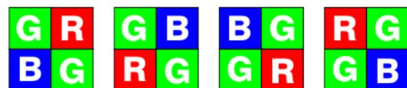
Figure 1. The used types of CFA in RGB color space
