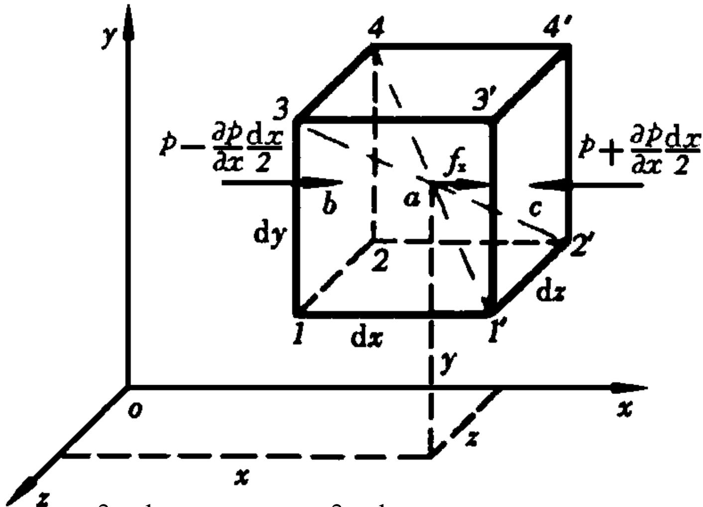
$$\left(p - \frac{\partial p}{\partial x} \frac{dx}{2}\right) dy dz - \left(p + \frac{\partial p}{\partial x} \frac{dx}{2}\right) dy dz + f_x \rho dx dy dz = 0$$
