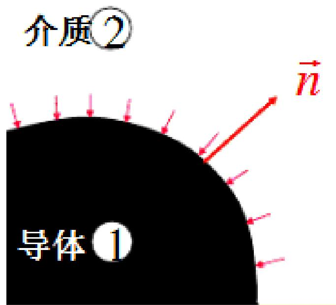
$$\left\{ \begin{array}{l} \phi = C \\ \epsilon \frac{\partial \phi}{\partial n} = -\sigma \end{array} \right. \quad (11)$$
