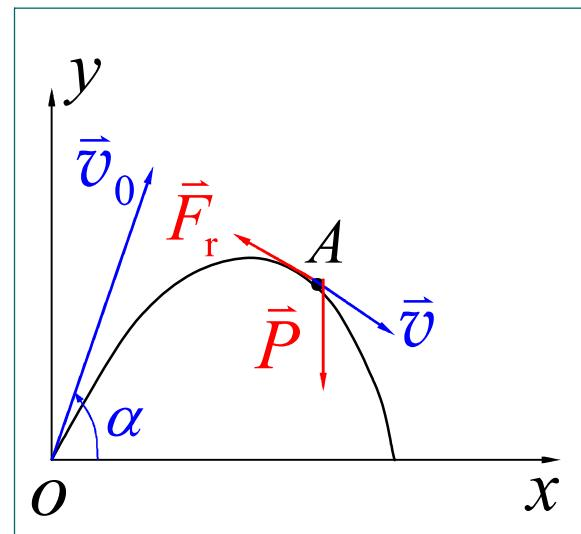
$$\left\{ \begin{array}{l} v_x = v_0 \cos \alpha e^{-kt/m} \\ v_y = (v_0 \sin \alpha + \frac{mg}{k}) e^{-kt/m} - \frac{mg}{k} \end{array} \right.$$
