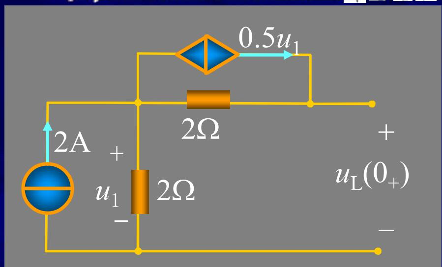
由 $0_+$ 电路模型:  $u_L(0_+) = 0.5u_1 \times 2 + u_1 = 2u_1 = 8V$
