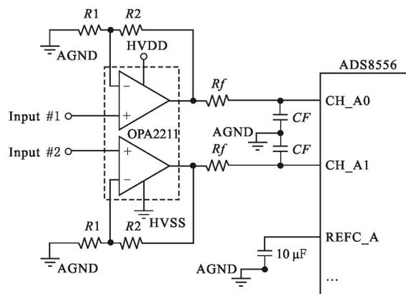
Fig.4 ADS8556 pre-conditioning circuit
