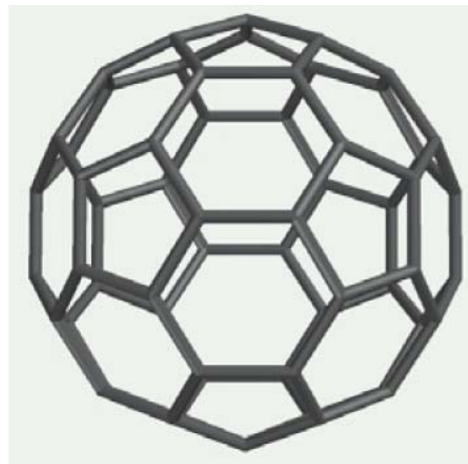
FIGURE 7.8 Buckminsterfullerene (C 60 ). Note that all carbons are equivalent and that no five-membered rings are adjacent to one another.
