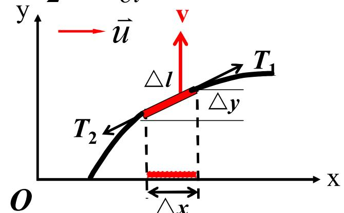
$$\approx \Delta x \left[ 1 + \frac{1}{2} \left( \frac{\partial y}{\partial x} \right)^2 \right] \quad W_p \approx \frac{1}{2} T \Delta x \left( \frac{\partial y}{\partial x} \right)^2$$
