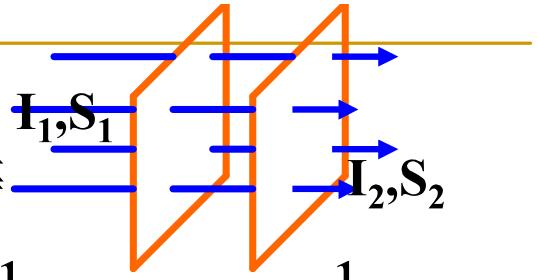
平面波  $I_1 S_1 = I_2 S_2$   $\rightarrow I_1 = I_2 = \frac{1}{2} \rho A^2 \omega^2 u = \frac{1}{2} \rho A^2 \omega^2 u$
