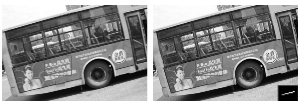
(a) Captured running bus image (b) Deblurred image and PSF path (in red box)
