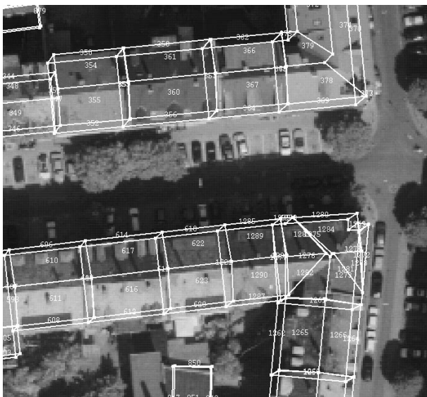
Figure 15: Reconstructed buildings projected into stereo image.
