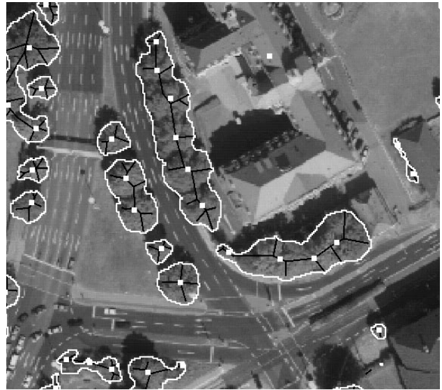
Figure 14: Computation of tree positions using the skeleton of the tree class segmentation result.
