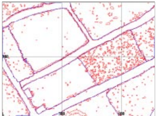
Figure 10: shows the object boundaries of the ground truth map (blue) superimposed to the improved maximum likelihood results (red)
