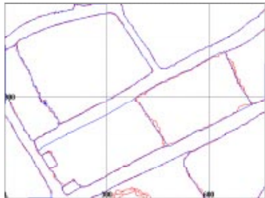
Figure 11: shows the object boundaries of the ground truth map (blue) superimposed to the likelihood-based classification results (red)
