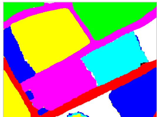
Figure 8: Shows the final result of likelihood-based classification. This Figure shows the result of local hypotheses testing resulting in a segmented image. Small segments have been removed and shape hypotheses initiated.
