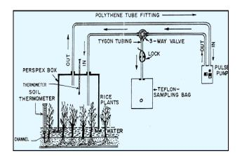
Figure 1. The Schematic Diagram Showing the Field Assembly of Methane Sampling Procedure
