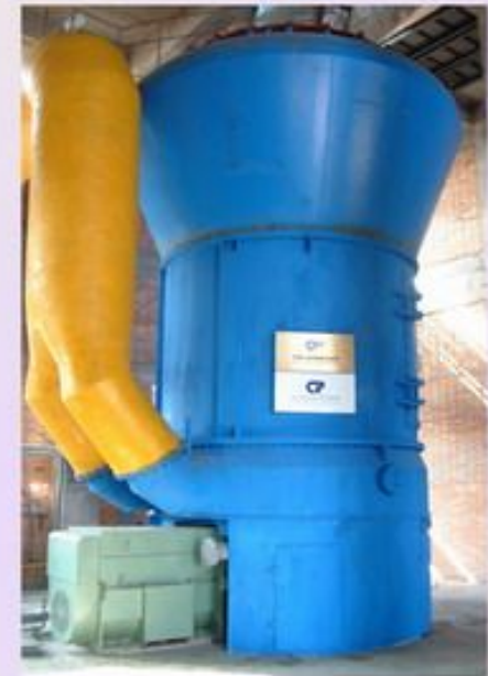
与德国CP公司合作的EM型磨煤机 EM COAL COOPERATED WITH CP IN GERMANY
