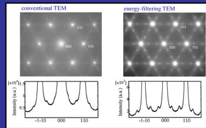
Energy filtering can also be used to improve diffraction patterns eliminating scattered, but not diffracted, electrons from the image. Like transmitted electrons diffracted electrons have no energy loss.
