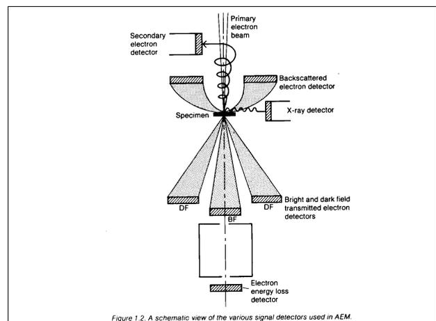
Figure 1.2. A schematic view of the various signal detectors used in AEM.
