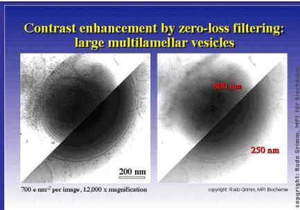
Zero-loss images are those created by only using the transmitted, and thus no energy loss, electrons. They have increased contrast due to the elimination of scattered electrons but retain high resolution because an objective lens aperture is not needed to eliminate scattered electrons.
