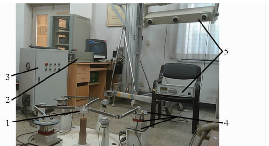
图11 含有柔顺关节的平面并联机器人实验系统 Fig. 11 Experimental system of planar parallel robot with compliant joints
