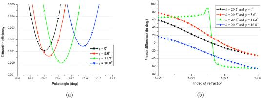
Fig. 2. (a) Diffraction efficiency as a function of polar angle for given azimuth angles. (b) Phase response for different incident angles.
