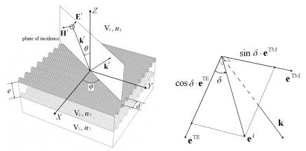
Fig. 1. Schematic representation of diffraction by a layered metal grating and definition of the polarization angle.
